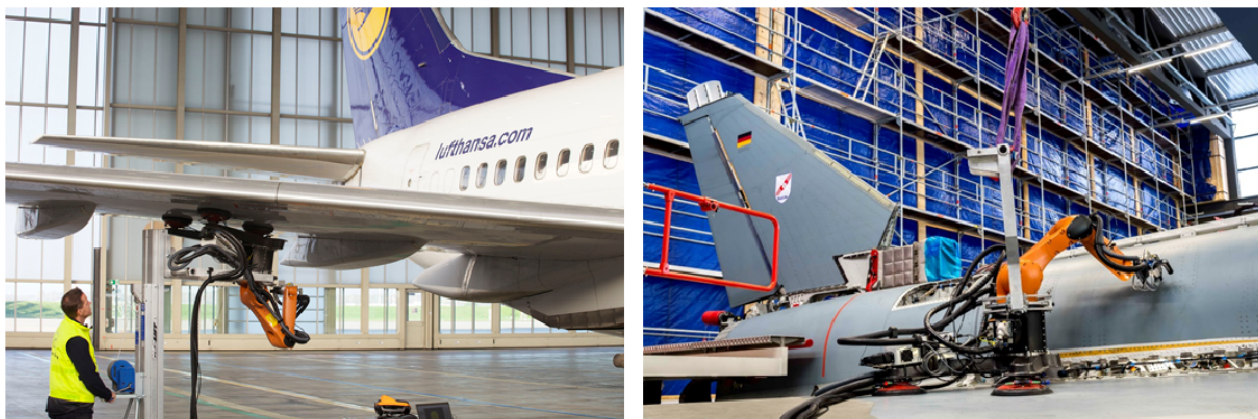
Figure 4: Robotic scarfing system
